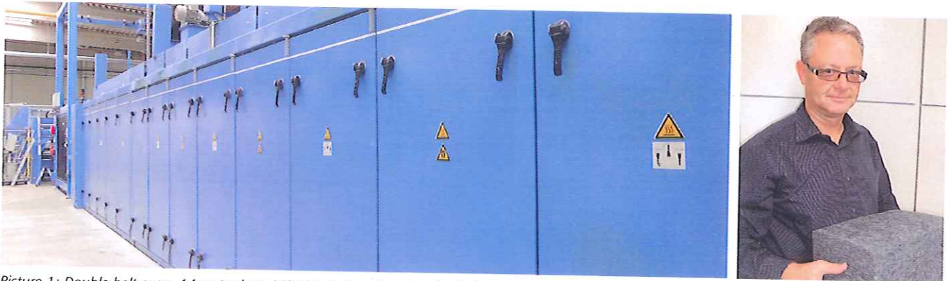
Picture 1: Double belt oven, 14 meter long / Picture 2: Uwe Rudolph, Technical Director of Ziegler Group
