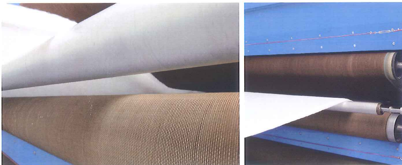
Double-Belt Dryer with non-stick-coated lower belt and magnetic upper belt from GKD
