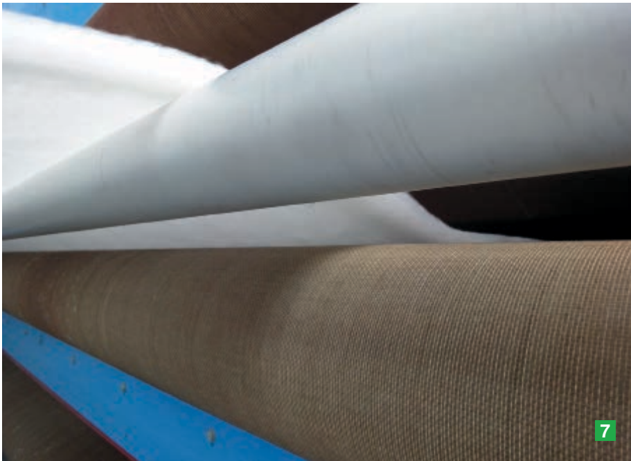
Fig. 7-8: Made-to-measure dryer belt from GKD meets the special requirements of the thick insulation products.
